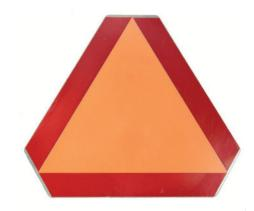
Per Kansas law, a Slow Moving Vehicle must have a triangularshaped emblem of substantial construction having equal sides of 14 inches and an altitude of 12 inches. shall be painted a fluorescent yellow-orange color and bordered with reflective red-colored strips having a minimum width of 1¾ inches. (Reference: Kansas Statutes, K.S.A. 8-1717)
