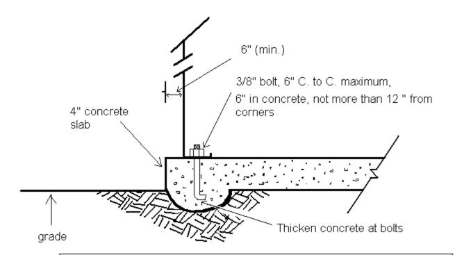
FOUNDATION RECOMMENDED FOR MANUFACTURED METAL ACCESSORY BLDGS. 160 SQ. FT. OR LESS. NO PERMIT REQUIRED FOR BLDGS. 120 SQ. FT. OR LESS.
